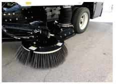
Dust suppression spray nozzles located at front, brooms and pick-up head
